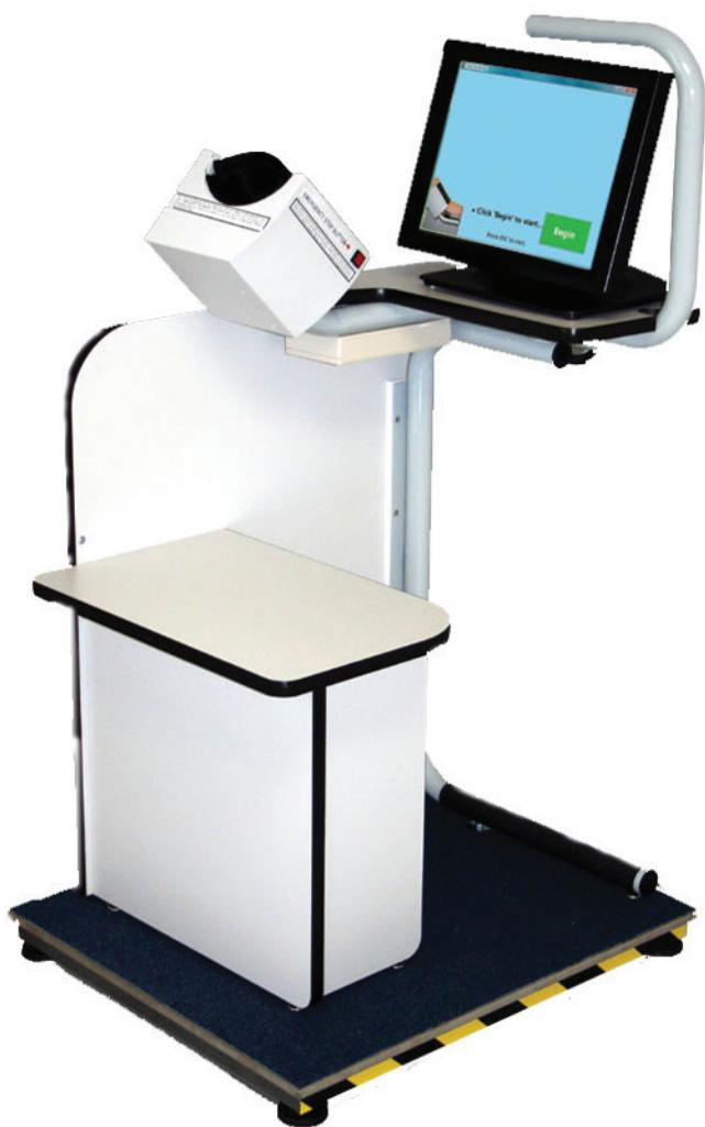
The **blood pressure measurement** fully satisfies specifications ANSI/MMI SP-10:2002 and incorporates a unique cuff that wraps around the arm similar to how a doctor measures blood pressure. This has advantages over the rigid tube approach that limits maximum arm size to what would fit in the tube. Moreover, for small diameter arms, the HealthGuard method does not require the bladder to hyper-inflate thereby causing a loss of sensitivity in the measurement.
